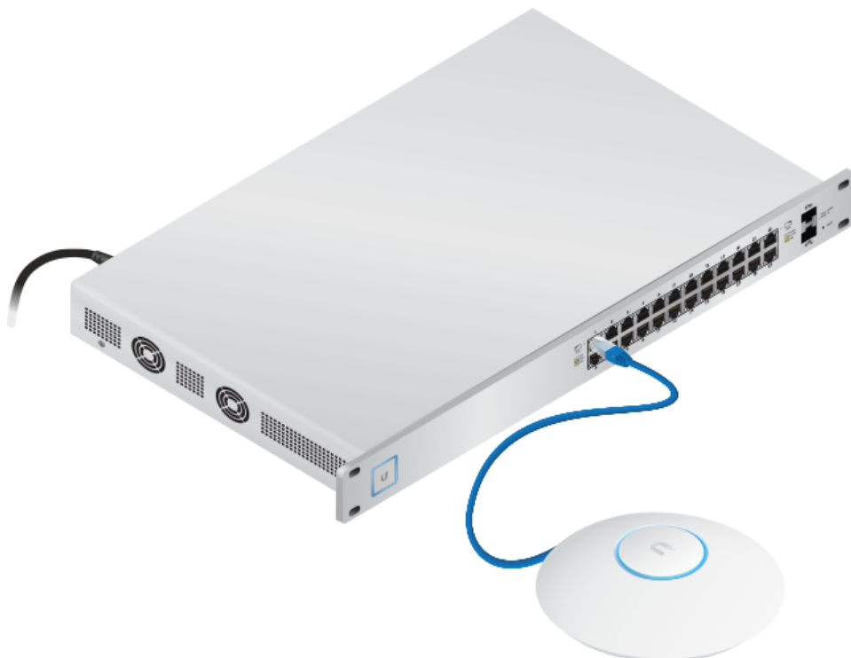
UniFi Switch with PoE Power Connection Diagram
